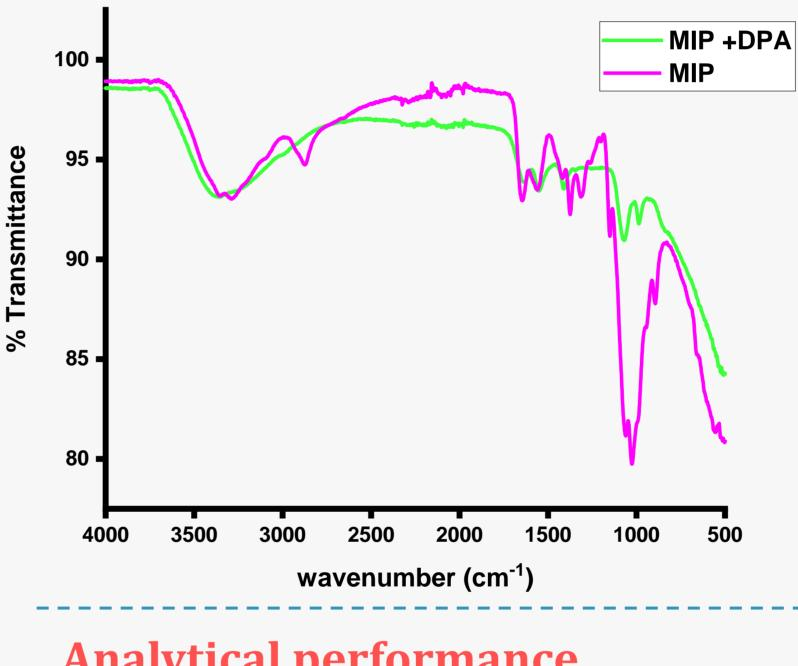
FTIR spectra of the synthesized MIP before and after the addition of DPA. The disappearance of the 2 over 3000 cm<sup>-1</sup> peaks and formation of 1 broad peak prove the formation of hydrogen bonds between chitosan and DPA.
