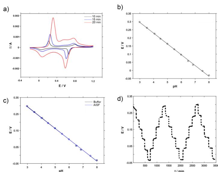
**Figure 2.** Electrochemical characterization and analytical performance of the SNGC-PANI sensor: a) resulting cyclic voltammety obtained with different electrodeposition times, ranging from 10 to 20 min, b) calibration curve of the pH sensor SNGC-PANI obtained ranging pH from 3-8, c) performance comparison between buffer and artificial interstitial fluid (AISF) media, d) potentiometry obtained for the reversibility assays ranging pH from 3 to 8.
