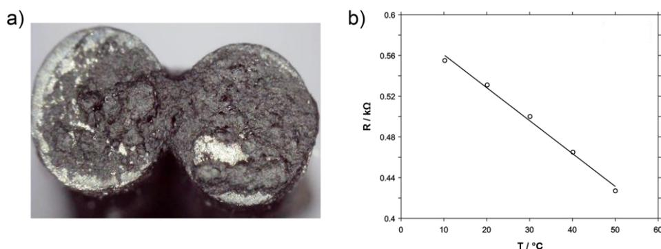
**Figure 3.** Optical characterization and analytical performance of the temperature based on SNGC-MWCNTs: a) optical microscopy with 1000x magnification factor, b) calibration curve of the temperature sensor SNGC-MWCNTs.
