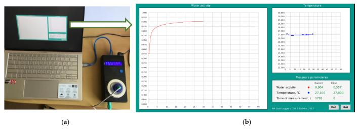
**Figure 2.** An Arduino-based water activity data acquisition device of foodstuff: (a) Photograph of a device connected to a computer; (b) Screenshot of the user interface for monitoring the change in water activity and temperature over.
