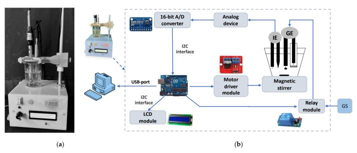
**Figure 3.** An Arduino-based water activity data acquisition device of foodstuff: (a) Photograph of the device; (b) A general Arduino-based circuit for constant-current coulometric titration equipment with potentiometric indication of the titration end point.
