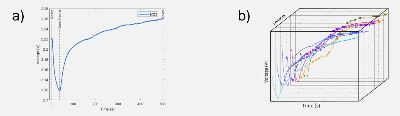
Figure 2. a) The response a white tea detects of sensor MQ3. b) The 3d-representation of one sample
