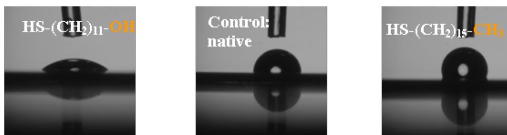
Figure 1. Variation of the contact angle according to the structure of the adsorbed thiol
