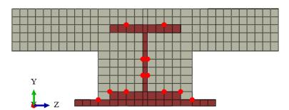
Figure 4. Distribution of connecting elements along the cross section of the FE model.
