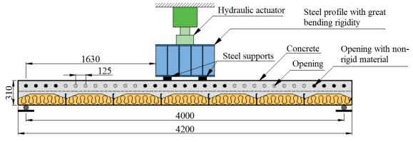
Figure 2. Structural configuration used by Braun et al. [6].
