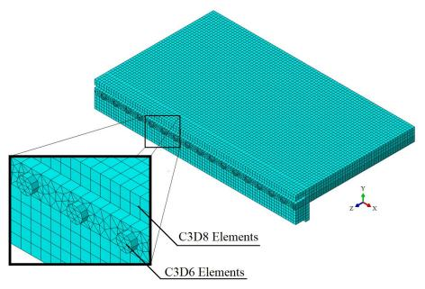
Figure 3. Mesh used in FE models and detail of the opening region (concrete dowel).
