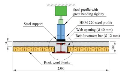
**Figure 1.** Geometric characteristics of the prototypes B1, B2, S1 and S2 experimentally tested by Braun et al. [6].
