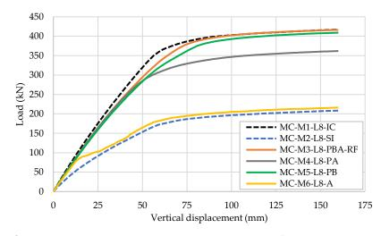
**Figure 6.** Load vs. vertical displacement curves obtained from FE models with different connection mechanisms.
