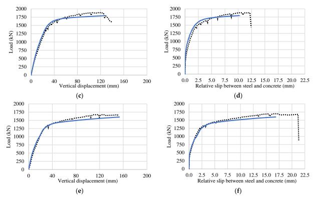
**Figure 5.** Comparison between experimental (dotted black lines) and numerical (solid blue lines) results. (**a**,**b**) prototypes B1 and B2; (**c**,**d**) relative load vs. slip results of prototype S1; and (**e**,**f**) prototype S2.
