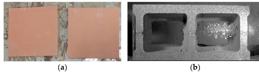
**Figure 2.** Samples used in ballistic penetration tests: (a) Clay slabs, (b) Concrete blocks.
