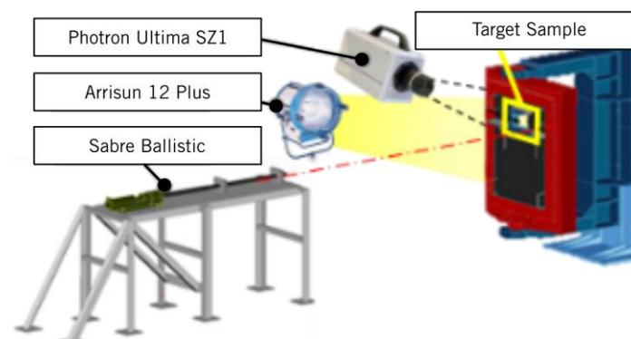
**Figure 3.** Testing device.
