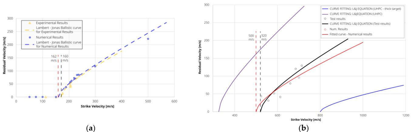
**Figure 5.** Comparison of the results obtained by numerical models with respect to the ballistic impact tests. (a) for clay (b) for concrete blocks.
