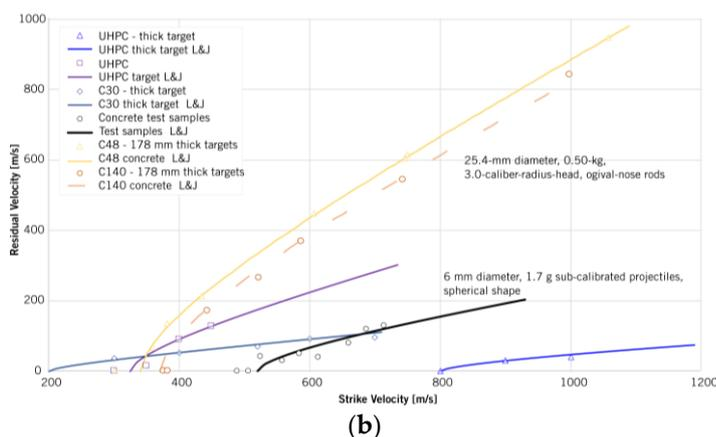
**Figure 1.** Comparison of curves obtained using own generated numerical models using JH-2 parameters from the literature compared with the curve obtained performing penetration tests. (a) for two batches of glass (b) for concrete.
