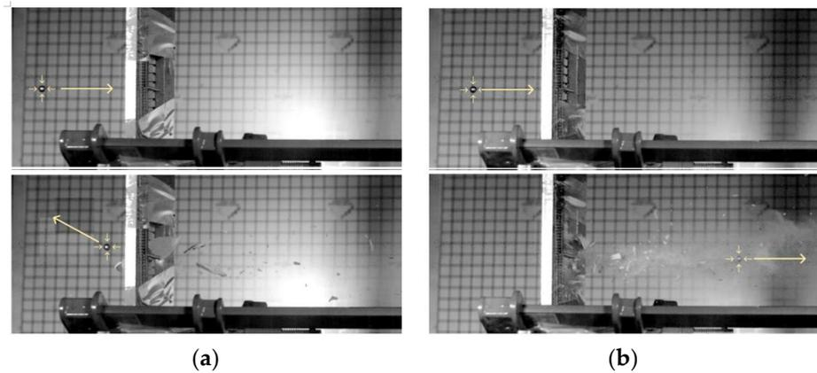
**Figure 4.** Impact tests. (a) Impact at 111 m/s: projectile rebound. (b) Impact at 205 m/s. penetration and debris clouds of material.
