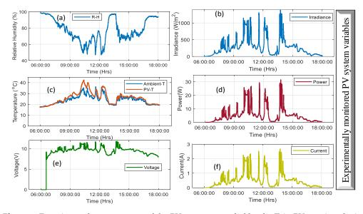
**Figure 7.** Experimental measurement of the PV system recorded by the Trio-PV-monitor devise on a 30 W PV system, 3 September 2023. (a) Relative Humidity (b) Irradiance (c) Ambient Temperature and PV Temperature (d) system Power (e) System Voltage (f) System Current.
