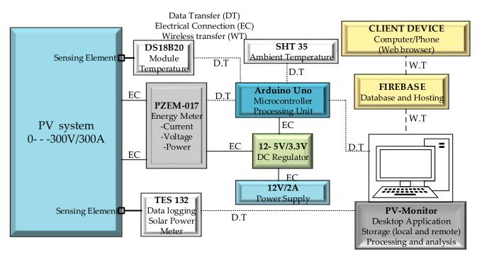
Figure 1. Conception block diagram of the Trio-PV-Monitoring system.
