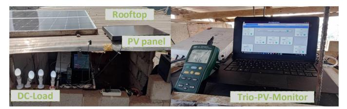
Figure 5. Trio-PV monitoring system in operation.
