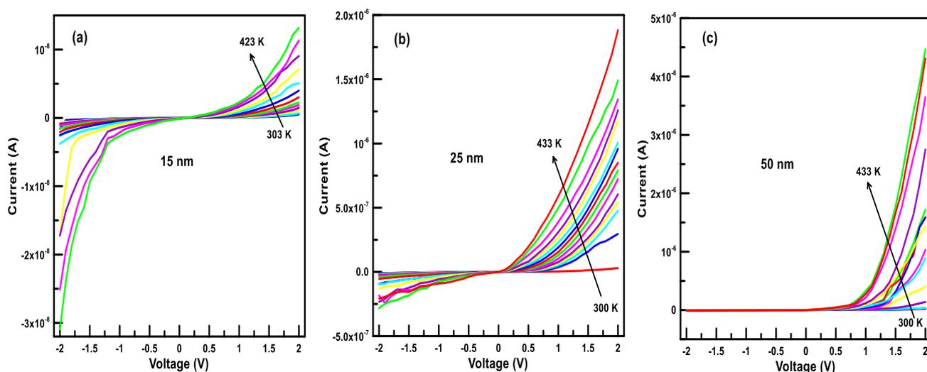
**Figure 2.** I-V characteristics of EuS thin films of different thicknesses: 15 nm (a), 25 nm (b) and 50 nm (c)
