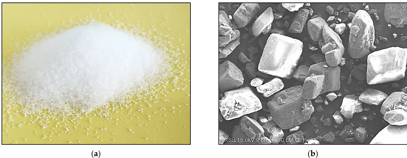
Figure 2. (a) Photo and (b) SEM image of the retarder employed in the present study.
