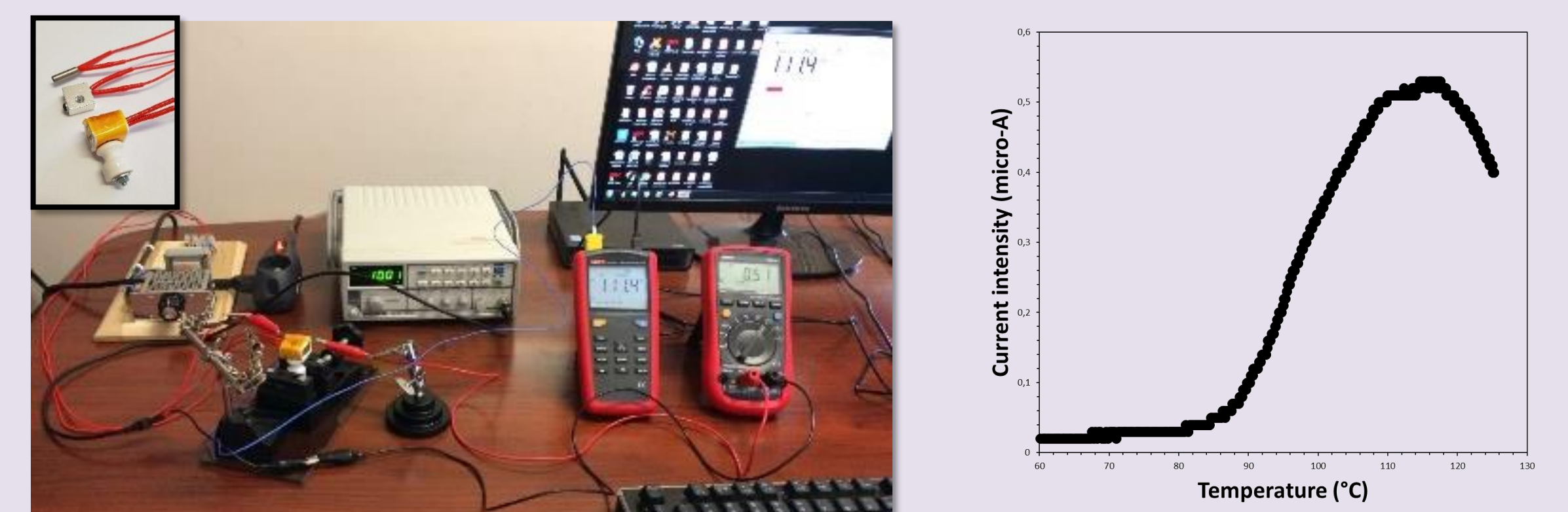
Figure 7. Experimental setup used for the calibrated temperature tests (a) and obtained I_{eff} - T curve (b).
