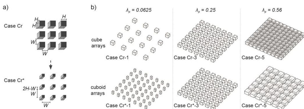
**Figure 1.** Two groups of block arrays investigated in this work; (a) diagram of the form types;  $H$ : building height;  $W$ : distance between buildings; (b) sketches of example subcases;  $\lambda_p$ : planar area density.
