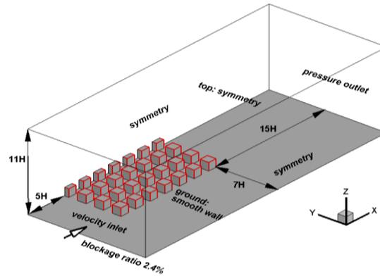
Figure 2. Computational domain setting following the AIJ guidelines.
