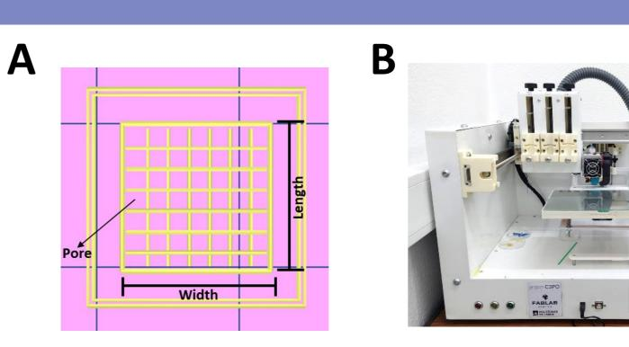
**Figure 1.** Scaffold CAD model (1 x 10 x 10 mm) **(A)** and Regemat 3D Bioprinter **(B)**.
