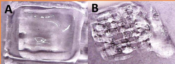
Figure 3. Scaffolds printed with 2.0 wt% (A) and 2.5 wt% (B) of chitosan.
