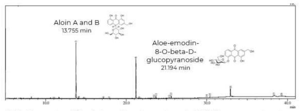
HPLC, Nexera system (Shimadzu), consisting of an autosampler SIL-30AC, a mass spectrometer QExactive Plus; Explice Plus C-18 column (150 mm  $\times$  3 mm, 3.5  $\mu$ m film thickness), flow 0.4 mL/min. The column oven was thermostated at 40°C. The solvent is methanol with 2% acetic acid. MS scan range of m/z 100 to 1500 amu.
