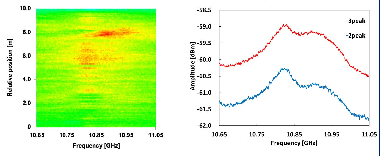
In both experiments, BFS at heated section (~8 m) shifted to higher frequency
