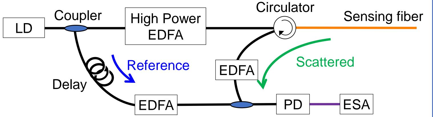
LD: laser diode, EDFA: erbium-doped fiber amplifier, **PD**: photo detector, **ESA**: electrical spectrum analyzer
