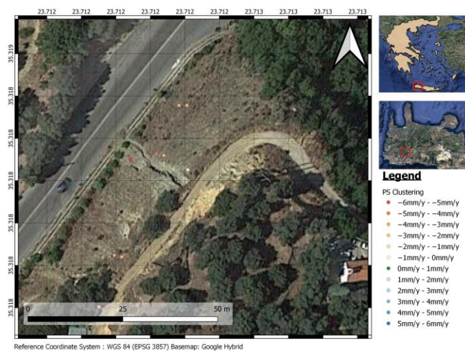
Figure 2. Identifying a landslide using P-PSI method
