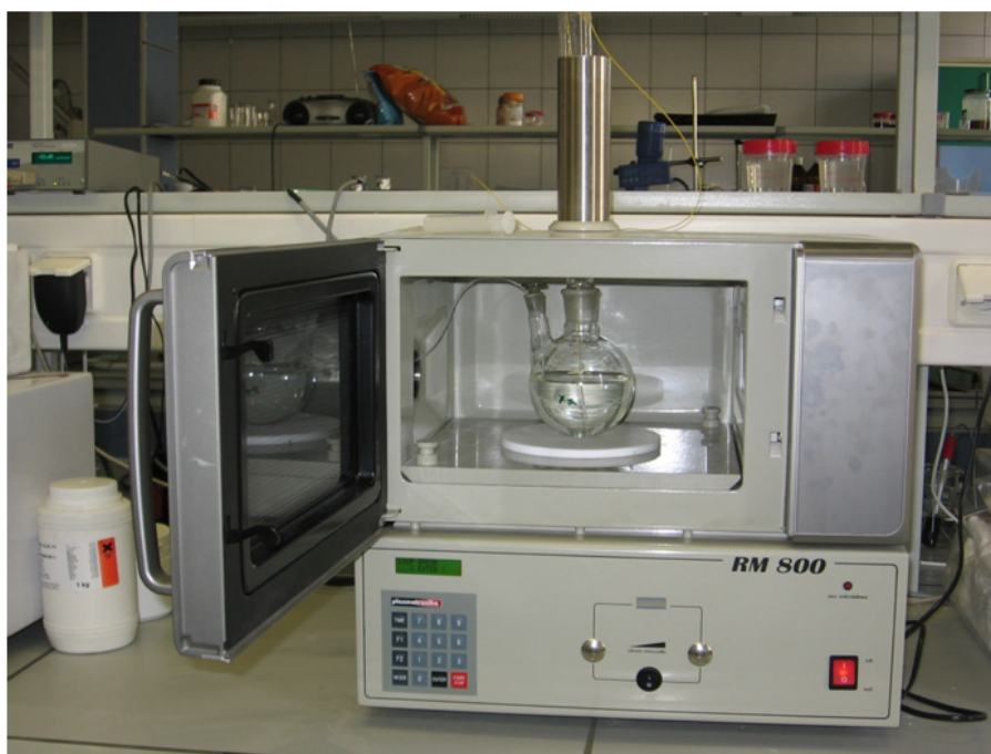
Figure 1: RM-800 microwave reactor (Plazmatronika, Poland)
