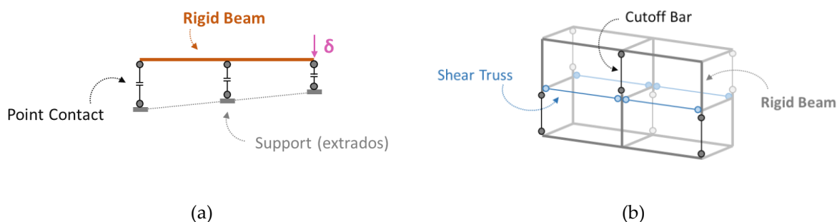
Figure 3: (a) scheme of the load pattern for load distribution; (b) scheme of the shear resisting joint.
