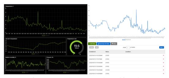
Figure 2. An example of a dashboard (user's front end, left) and a feed (developer's back end, right) on Adafruit IO.
