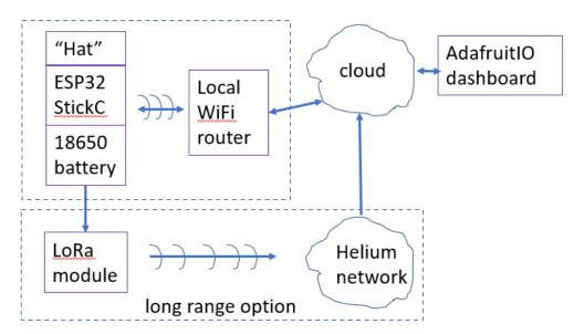
Figure 1. Block diagram of the hardware setup and wireless connections that were fully prototyped.
