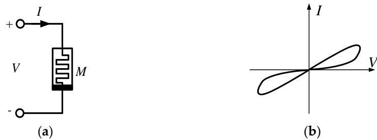
Figure 3. The Memristor [7]: (a) Symbol; (b) The I - V characteristic curve.
