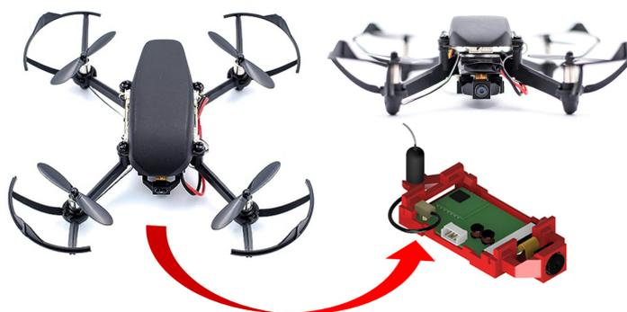
Figure 4. Drone with WiFi Camera Module.
