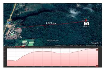
**Figure 4.** Validation Route for LoRa Communication Distance Between Gateway and Device, and Terrain Elevation Profile.
