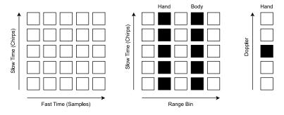
**Figure 1.** Illustration of the reduced 1D radar processing algorithm. Raw radar is illustrated data for one antenna (**left**). The hand and the body are resolved with a discrete Fourier transform along the
