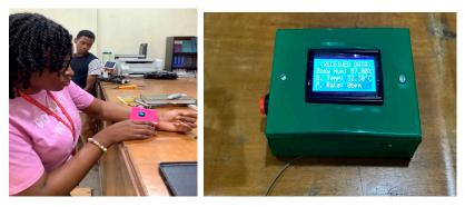
**Figure 4.** The use of the vitals monitoring prototype at the transmitter which is also displayed at the receiver end.
