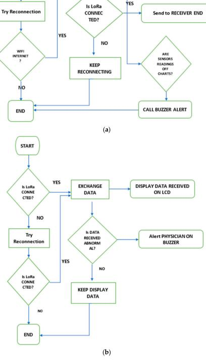
Figure 3. (a). Flowchart for LoRa Transmitter Circuit; (b). Flowchart for LoRa Receiver Circuit.
