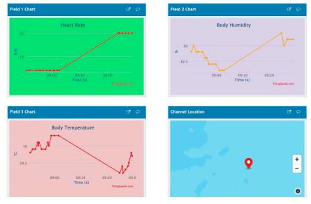
**Figure 5.** The ThingSpeak IoT platform showing pulse rate, humidity and temperature monitoring in real time. This data can be accessed from anywhere by the medical doctor of the patient.
