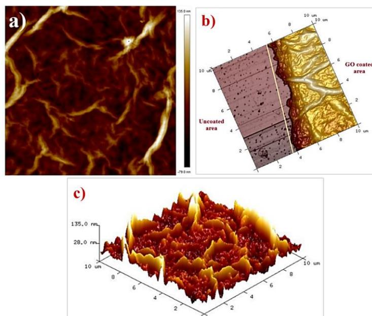
**Figure 5.** (a) 2D topography of AFM images of GO, (b) 3D AFM images of GO and (c) 3D AFM topography images of the boundary region between the uncoated and coated fibers of GO.
