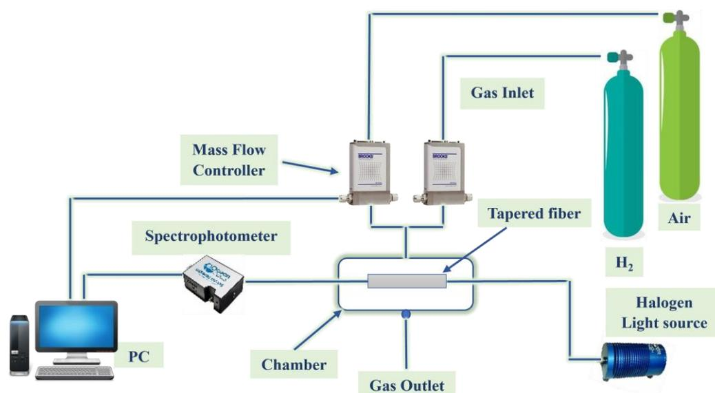
**Figure 2.** The experimental installation of the  $\text{H}_2$  sensor.
