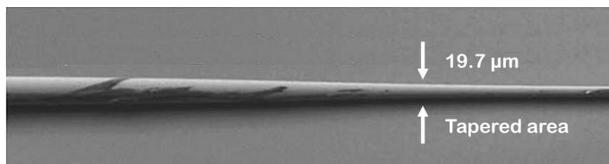
**Figure 1.** FESEM image of tapered multimode optical fiber (MMF).
