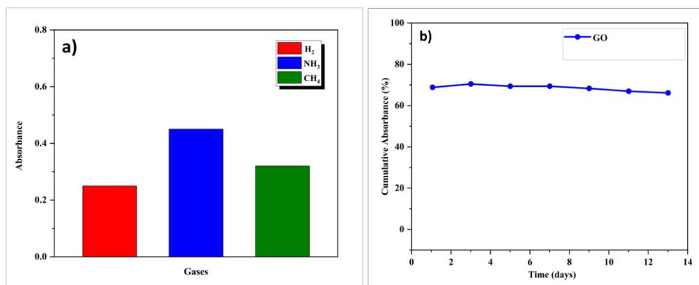
**Figure 7.** (a) Comparison bar graph of the selectivity of optical fibers coated with GO based sensor and (b) Stability of the GO based sensor.
