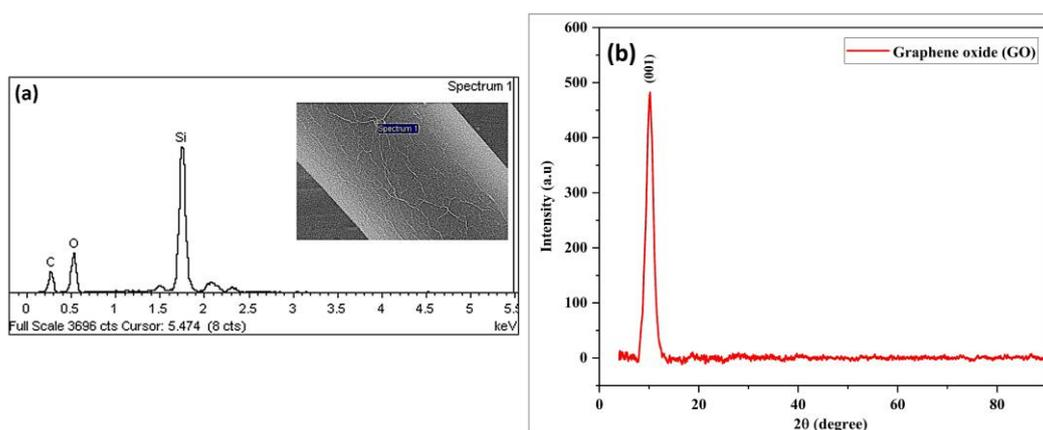
**Figure 4.** (a) EDX measurement of GO and (b) XRD pattern for both samples GO thin film.
