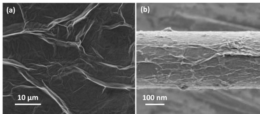
**Figure 3.** FESEM micrographs of tapered MMF coated with graphene oxide (GO).
