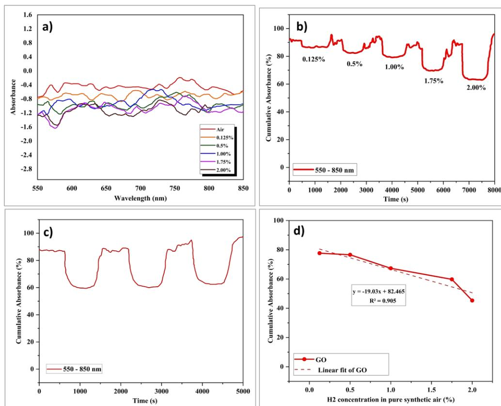
**Figure 6.** (a) GO Absorbance versus optical wavelength, (b) Dynamic absorbance curves of sensors coated with GO (c) The repeatability of the developed sensor and (d) Absorbance changes at different H<sub>2</sub> concentrations for coated GO.
