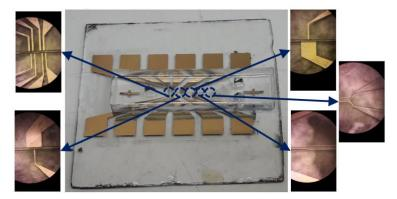
Figure 6. Fabricated chip structure.
