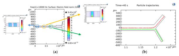
**Figure 4.** Optimized structure, (a) Electric field distribution (b) Particles' trajectory near the outlets.
