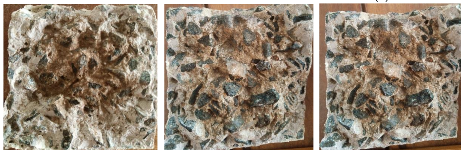
Figure 2. Extent of chloride ion penetration (into concrete specimens exposed to 3% NaCl) indicated by white precipitate of AgCl on outer layers of specimen.
