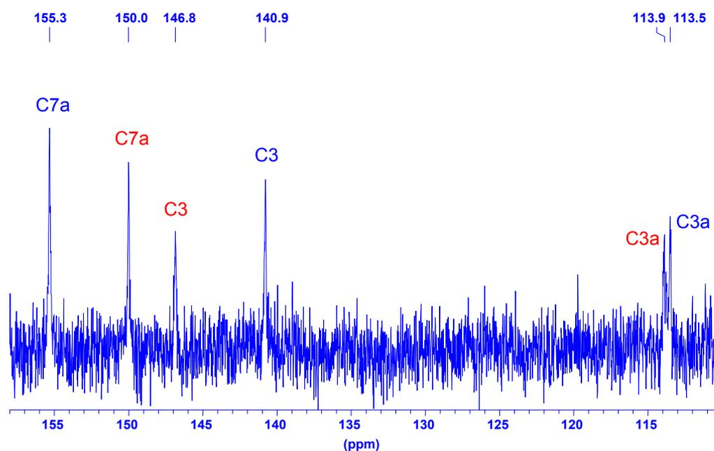
**Figure 1.** <sup>13</sup>C NMR spectrum (aromatic region) of compound **4** in DMSO-*d*<sub>6</sub> at 298 K
