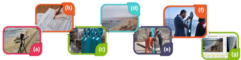
Figure 2. Workflow CoastSnap implementation in Valparaíso region, Chile. (a) Selection of the installation sites; (b) request for permits to install the platforms to the councils; (c) design, signaling, and construction of the platforms; (d) control points with GPS (e) installation of the platforms; (f) inauguration and start-up and (g) Extraction and processing of shoreline, from open-source code. .
