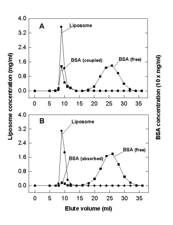
**Fig. 4.** Elution profiles obtained following coupling of modified BSA to the surface of MPB-LUVs. Liposome were monitored using a radiolabeld cholesteryl hexadecyl ether  $[^{3}H]CHE$ , and BSA protein was determined by the dansyl fluorescence intensity at 515nm, bandpass 8nm (excitation at 353, bandpass 2nm). (A). coupling reaction with MPB-liposome; (B). control reaction with MPB-free-liposome.
