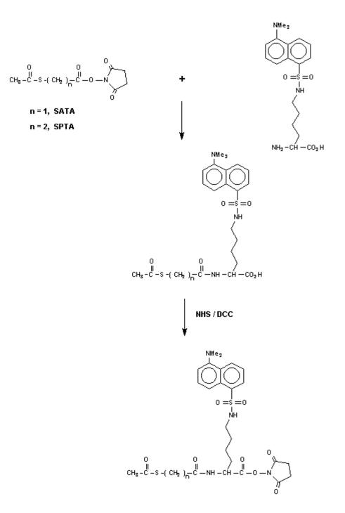
**Fig. 1.** Synthetic scheme for dansyl-labeled heterobifunctional fluoroscentcrosslinkers with NHS ester and acetyl protected sulfhydryl group.
