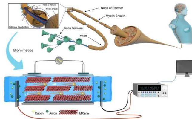
The neural saltatory conduction along axons is a unique action potential propagation pattern limited to myelinated axons, demonstrating ultrafast signal transmission. The bioinspired nervous signal transmission system is a 2D MXene nanofluidic device with signal input and acquisition modules, enabling real-time current feedback and signal transmission.
