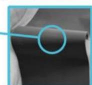
Each wedge tip, 1/100 of a human hair thickness, engage in shear using van der Waals force, not suction. A one square inch tile of our Dry Adhesive is covered in over 400 wedges that can hold 15 lbs. 6 tiles can pull a car!
