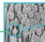
The unique geometry of our Dry Adhesive mimics the gecko's foot structure creating their signature no-residue grip. Our micro wedges replicate the soles of their feet that are covered in "hairs" called setae.
