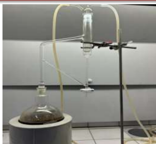
Hydrodistillation in Clevenger apparatus
