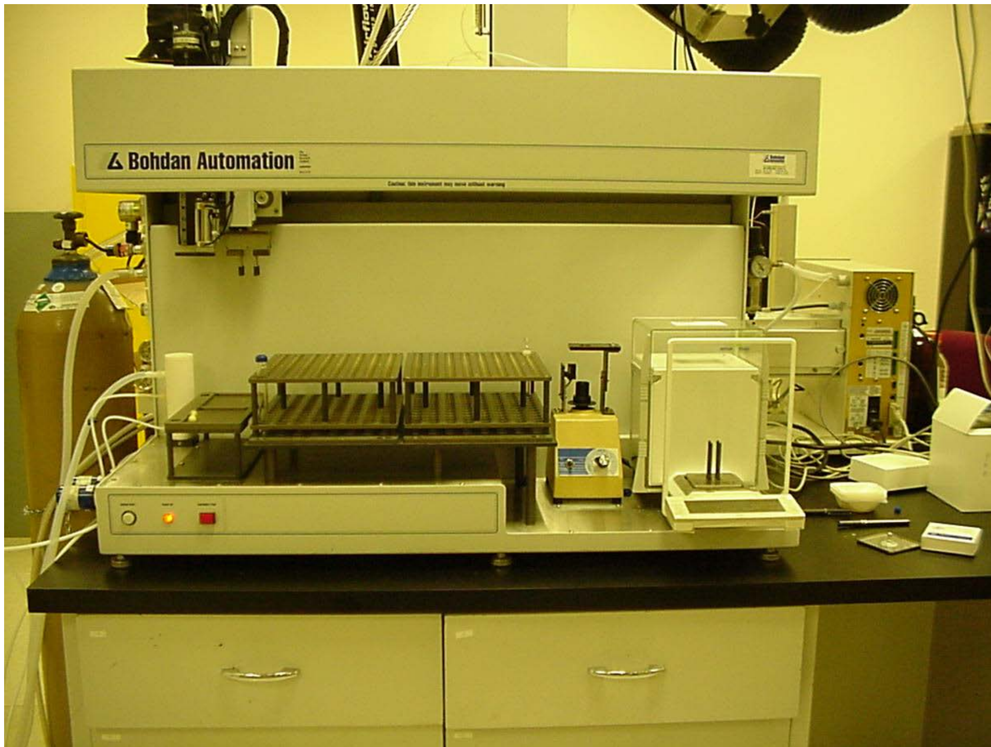
Figure 1. Bohdan weighing and dissolution station is used to make stock solutions of starting materials and reagents. Fitted with a balance, a vortex, and an arm equipped with cannula
