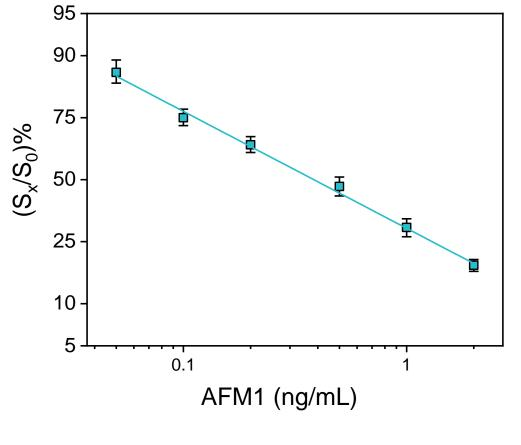
Real-time signal responses of calibrators containing  $0-2\ ng/mL$  in undiluted milk
