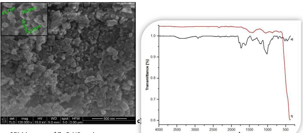
FTIR analysis for all samples exhibits a high-intensity band in the range 500–400 cm<sup>-1</sup>, which can be attributed to the vibration mode of the Zn-O bonds.
