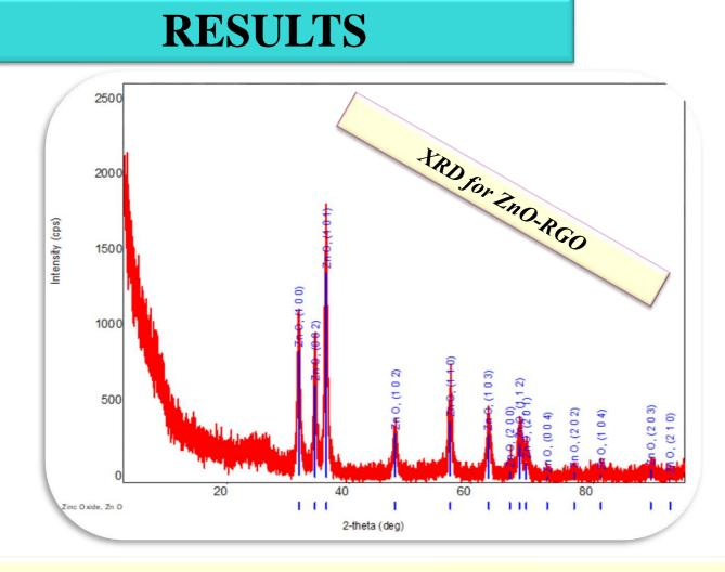
XRD structural analysis shows that the diffraction peaks can be attributed to ZnO wurtzite, with a slight shift of the peaks and a decrease in their intensity, indicating the insertion of oxide nanoparticles between the graphene sheets without changing the preferential orientation of the oxide.
