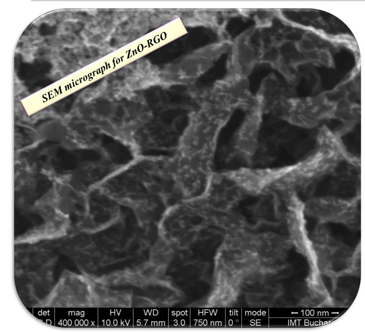
SEM images characteristic of ZnO-RGO composites show that ZnO nanostructured materials are distributed on the surface and embedded between the graphene sheets, showing good interaction between the components of the composites.
