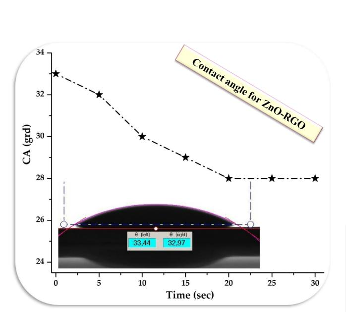
The contact angle is less than 90°, confirming that the obtained composites have hydrophilic surface properties.
