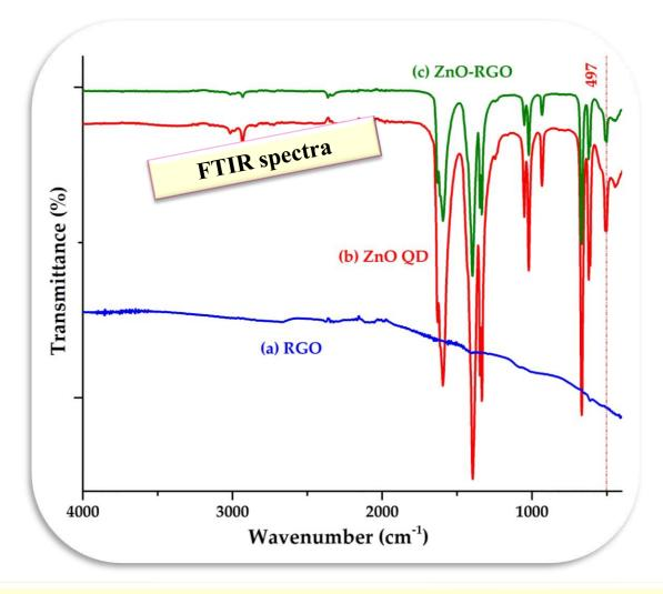
RGO does not show any IR absorption bands. The composite spectrum contains characteristic peaks of ZnO QD. A band associated with Zn-O can be observed at around 497 cm<sup>-1</sup>.
