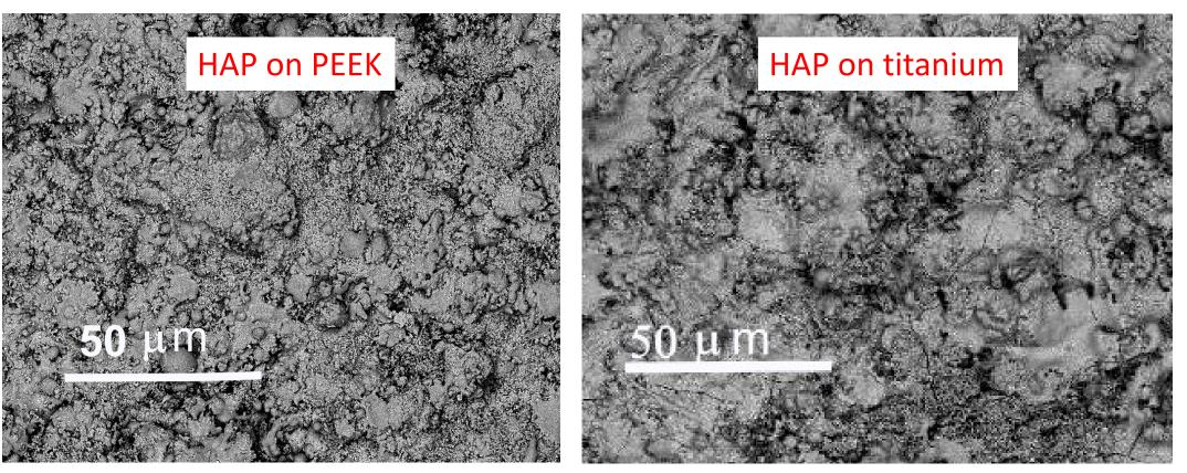
The SEM images of the surface of HAP coatings obtained using the GDD technique
