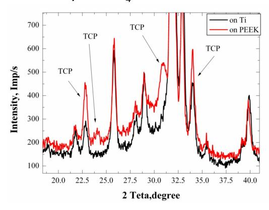
The diffractograms of HAP/PEEK and HAP/Ti coatings within the range of 20 – 40 degrees.
