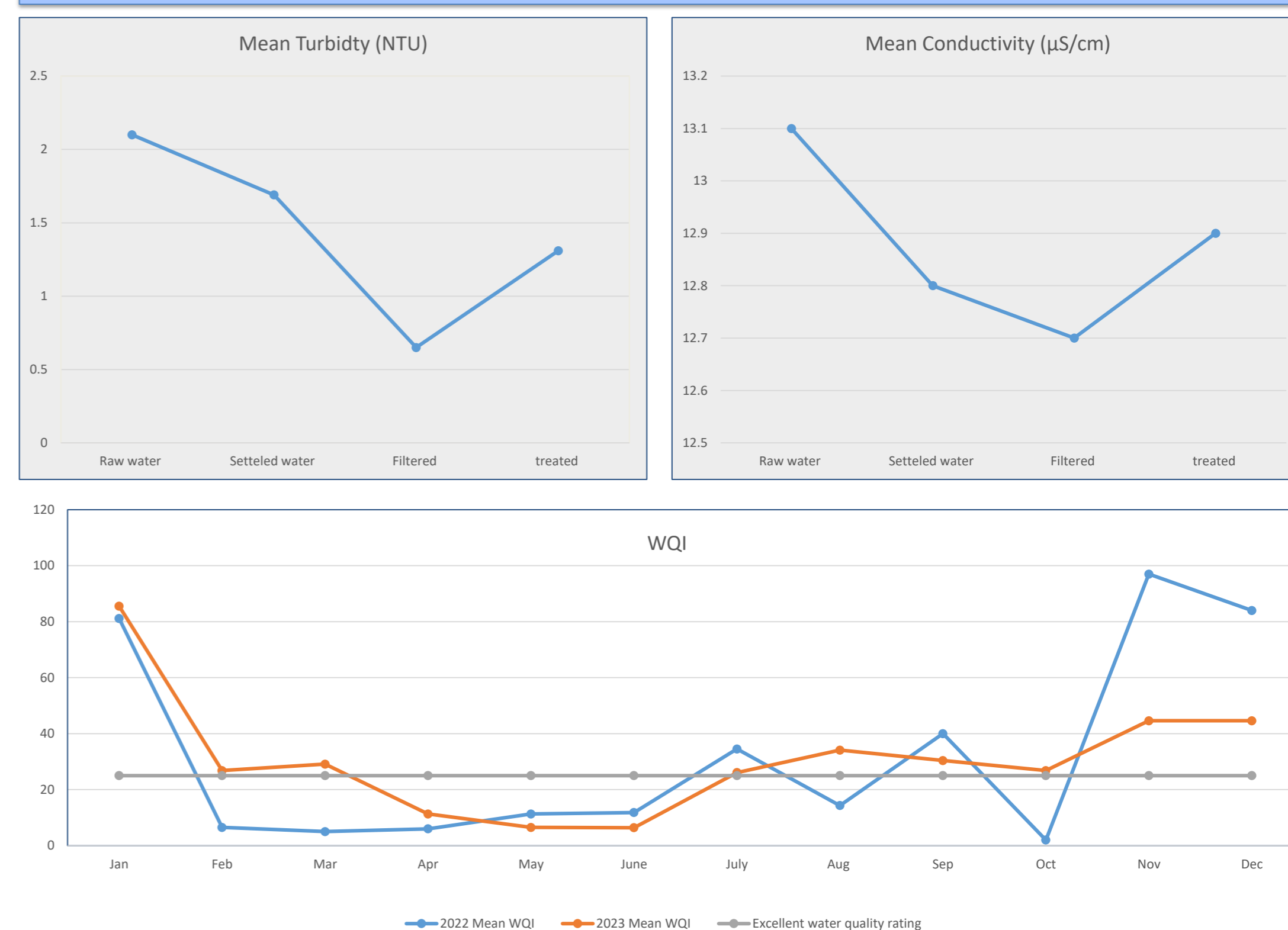
Figure 1: Variation of mean turbidity, mean conductivity along a treatment train and WQI for 2022-2023 data compared to the excellent quality rating.
