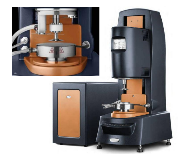
Force of Bioadhesion test (Mixing proteins with artificial saliva to simulate the oral environment)
