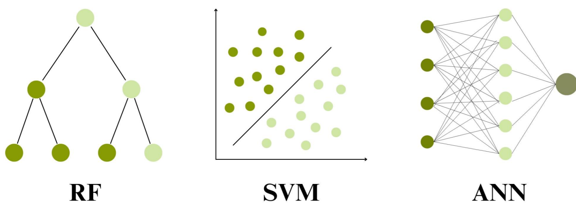
Figure 1. Machine learning algorithms; random forest (RF), support vector machine (SVM) and artificial neural network (ANN).
