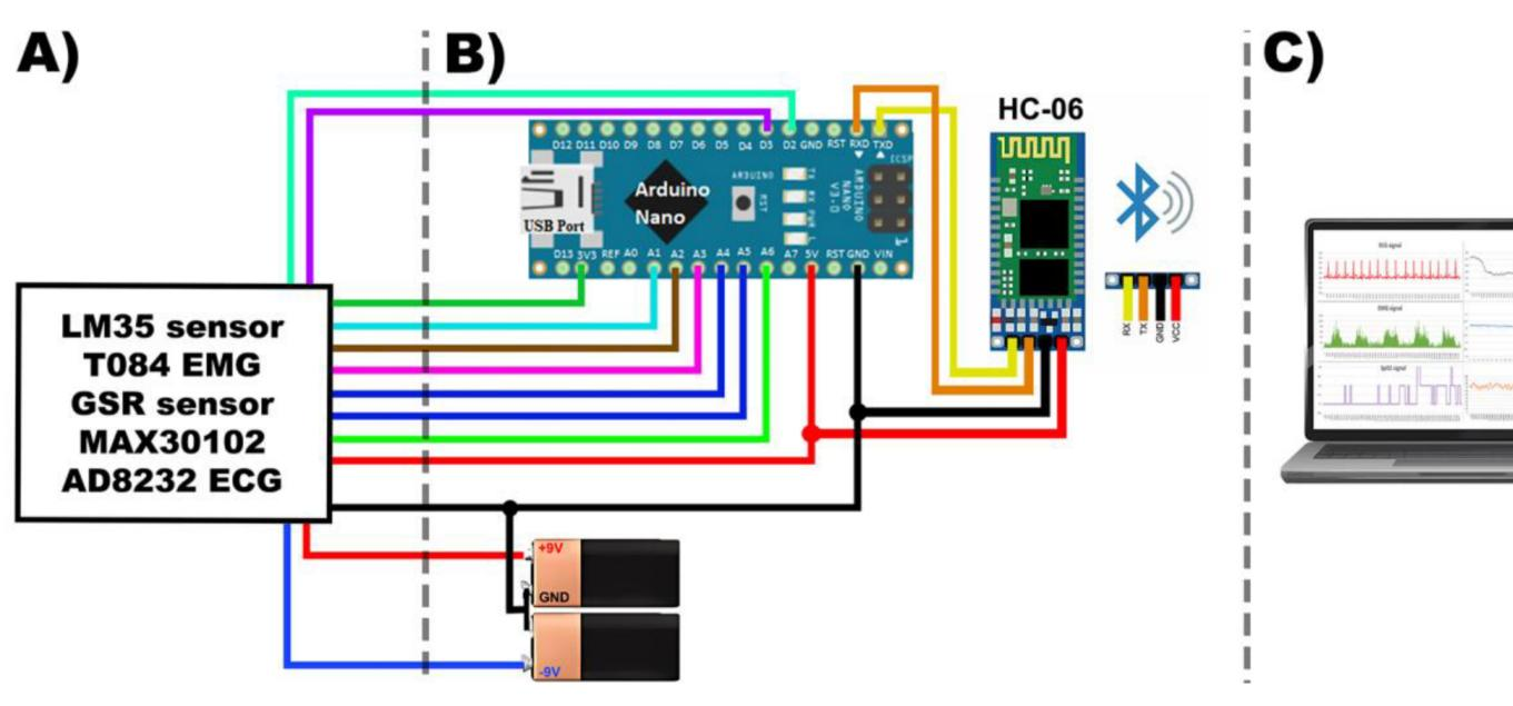
Fig. 1. Biosignal acquisition system connection diagram.
