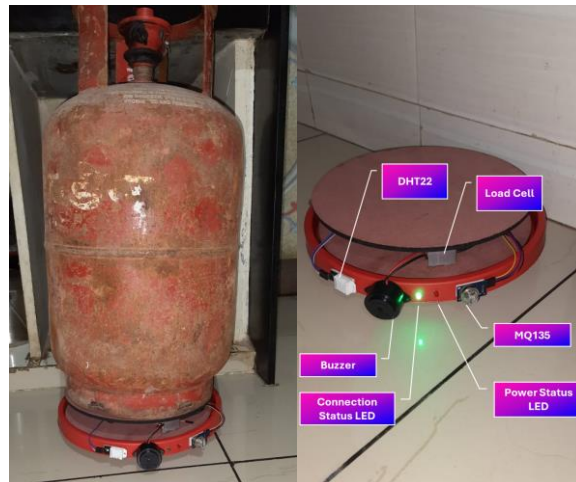
Figure 2. Real-time implementation of the proposed system.
