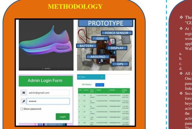
The solution for this problem is to develop a smart footwear with integrated sensor, GPS and modules to activate real time tracking and transfer of personal profile which contains Name, Photo, Mobile number, Working place of respective users to Control panel in case of force sensor is to ensure the women is safe and secure.
