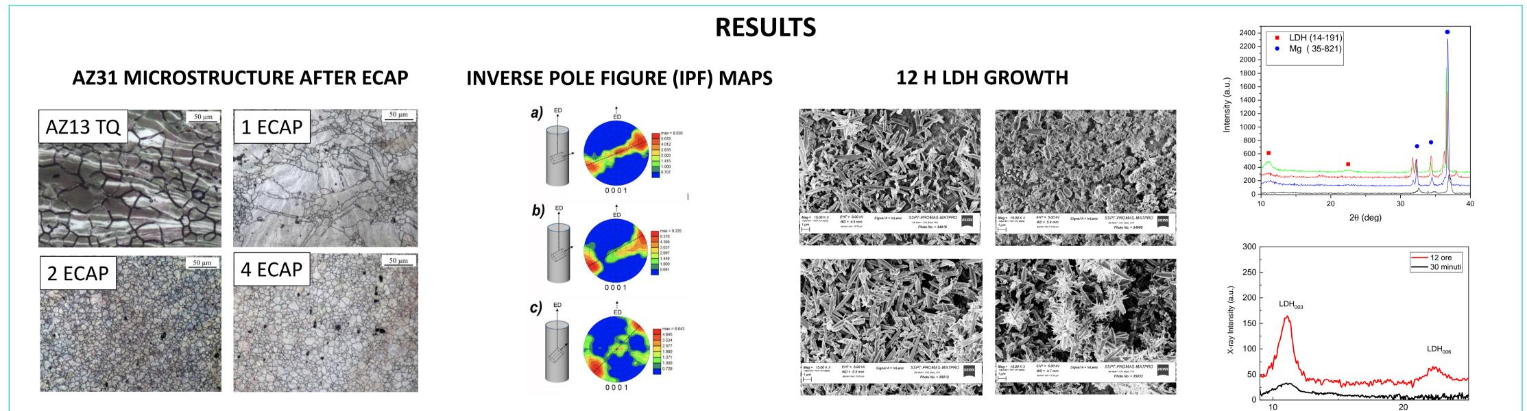
• All the samples are coated with LDH crystals with an elongated and dendritic morphology
