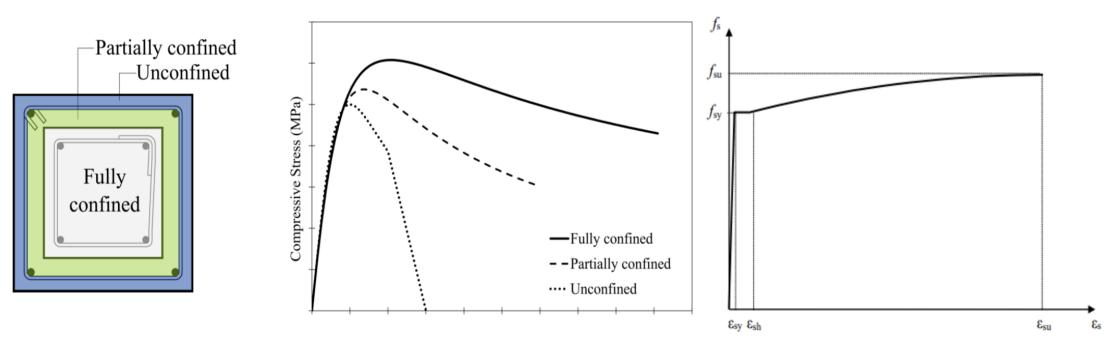
The code developed to estimate the moment-curvature relationship of jacketed RC columns was validated by experimental studies performed by Ersoy et al. (1993).
