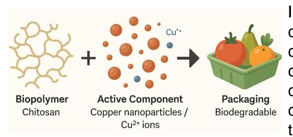
In this study, the bio-based polymer chitosan (CS), extracted from shells crustacean and insect cuticles, was functionalized with copper sub-microparticles. Both chitosan and copper are known for their antimicrobial properties,
