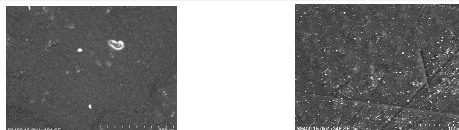
Figure 3. SEM image of NF membrane (left pristine (PEI/PSS) 5 , right: after MOF303 deposition
