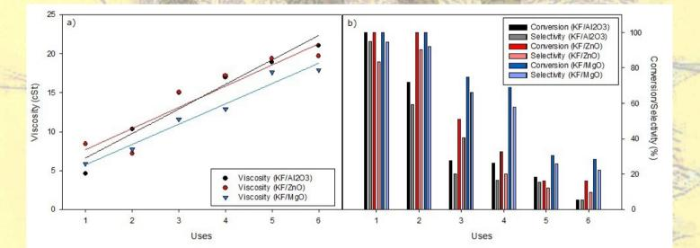
**Figure 6.** (a) Viscosity values obtained in the heterogeneous selective methanolysis of sunflower oil (viscosity 32.0 mm2/s) under standard conditions, with different catalyst, 0.8 g of catalyst, 12 mL oil, 2.43 mL methanol and 65 °C. (b) Conversion and Selectivity values obtained with identical conditions.
