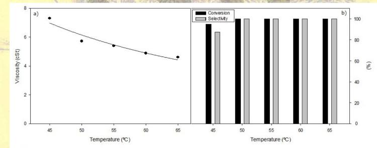
**Figure 4.** (a) Viscosity values obtained in the heterogeneous selective methanolysis of sunflower oil (viscosity 32.0 mm2/s) under standard conditions, with different temperatures (between 45-65 °C), 0.8 g of KF/Al2O3, 12 mL of oil and 2.43 mL of methanol. (b) Conversion and Selectivity values obtained with identical conditions.
