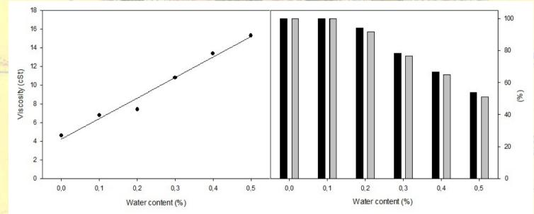
**Figure 5.** (a) Viscosity values obtained in the addition of water (from 0 to 0.5 % respect to the oil) in the partial methanolysis of sunflower oil (viscosity 32.0 mm2/s) under standard conditions, with 0.8 g of KF/Al2O3, 65 °C, 12 mL of oil and 2.43 mL methanol. (b) Conversion and Selectivity values obtained with identical conditions.
