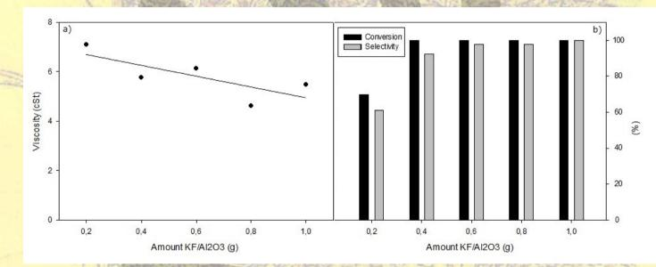
**Figure 2.** (a) Viscosity values obtained in the heterogeneous selective methanolysis of sunflower oil (viscosity 32.0 mm2/s) under standard conditions, with different amounts of KF/Al2O3, 65 °C, 12 mL of oil and 2.43 mL of methanol. (b) Conversion and Selectivity values obtained with identical conditions.
