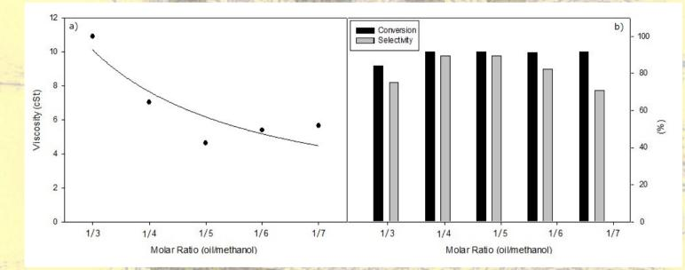
**Figure 3.** (a) Viscosity values obtained in the heterogeneous selective methanolysis of sunflower oil (viscosity 32.0 mm2/s) under standard conditions, with different molar ratio oil/methanol, 65 °C, 12 mL oil and 0.8 g of KF/Al2O3. (b) Conversion and Selectivity values obtained with identical conditions.
