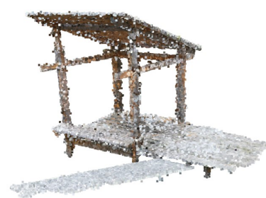
Figure 2. Filtered point cloud model of the architecture based on density-based spatial clustering of applications with noise (DBSCAN).
